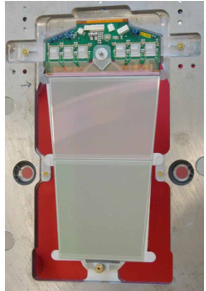
Module of current endcap strip detector
